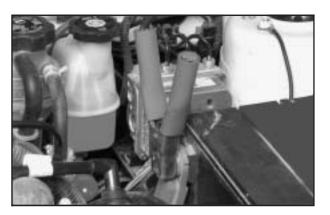
Connect the red positive (+) cable to the positive (+) terminal of the dead battery.
